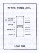
IMPORTANT: Holding the LOAD SIZE WATER LEVEL control lever in the RESET position can cause flooding of the washer.
